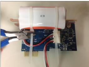
8. Zip tie second battery in place with wires going through the board gap. Pull the zip ties tight and cut off the excess. Rotate the buckles to the bottom.
