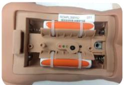
3. Cut all the battery wires near the battery end.
