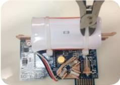
5. Disconnect the two battery connectors by pulling on the wires. ***Properly dispose of old batteries or return them to Realityworks.***
