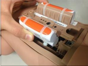
10. Secure the electronics assembly with two screws. Replace the back cover by inserting the Instructor Key, pressing down and turning 90 degrees clockwise.
