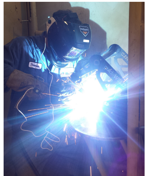
The guideWELD™ LIVE real welding guidance system being used as a training tool during live welding.
